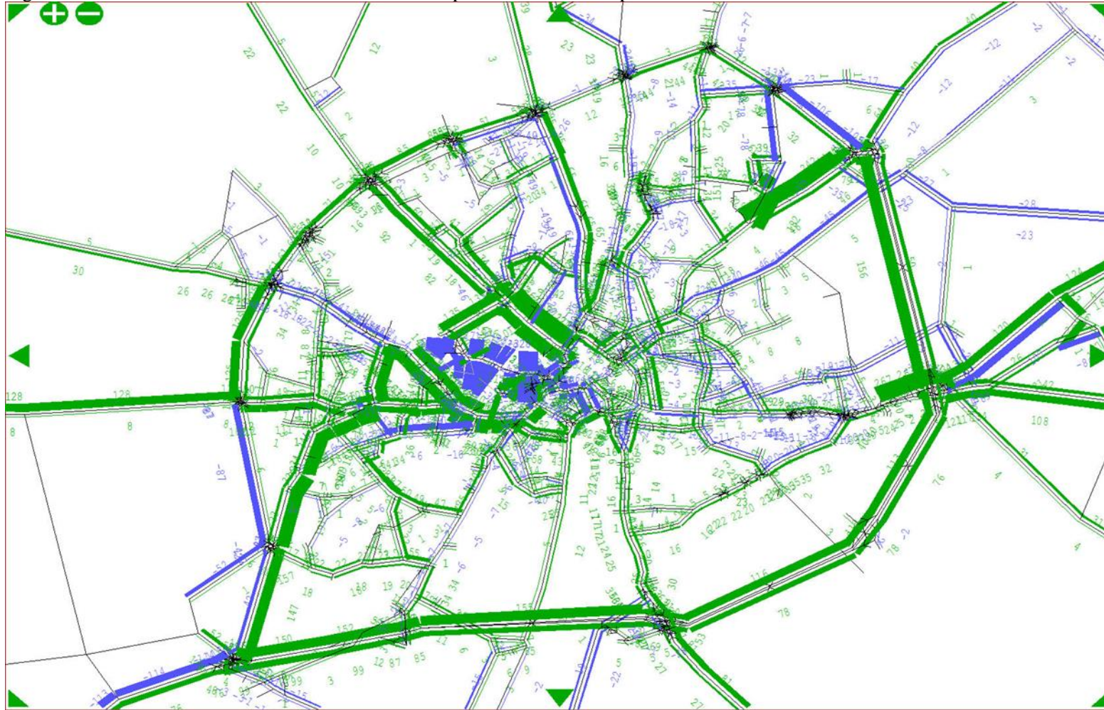
Figure D5: Link Flow Difference between DM and Option A – 2031 PM peak hour
