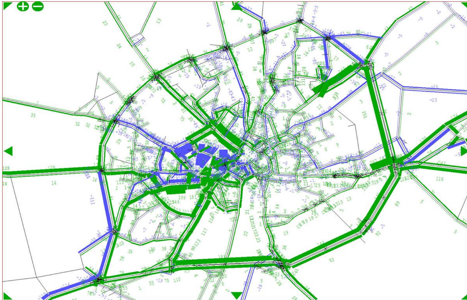
Figure D7: Link Flow Difference between DM and Option E – 2031 PM peak hour
